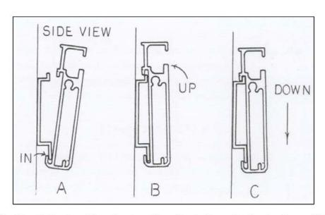
**STEP 2**: Attach the load bar by hooking the bottom to the bottom of the brackets (A), swinging the top into position over the top of the brackets (B), and then pushing down to establish a firm connection with the brackets (C).
