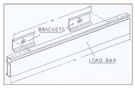
**STEP 1:** Position the Wall Mounting Brackets so that they are approximately 4" in from each end of the load bar that is to be attached. Firmly secure following the guidelines presented earlier.
